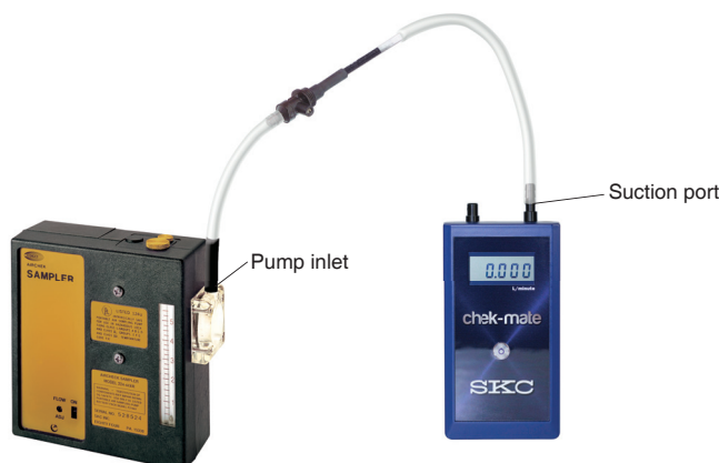
Calibration train with tube in adjustable tube holder
