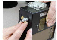
Thread exhaust port fitting into air discharge port on pump.
