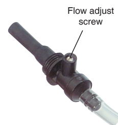
Figure 3. Single Adjustable Tube Holder with Sample Tube
